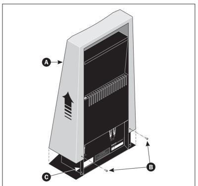
Figure 5: Mounting/Dismounting of the Cabinet
